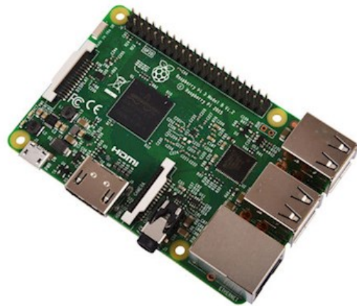
Figure 6: The Raspberry Pi 3B
